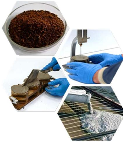
**Description:** Superplasticizer- a water soluble resin widely used as an admixture to enhance the fluidity of concrete.
